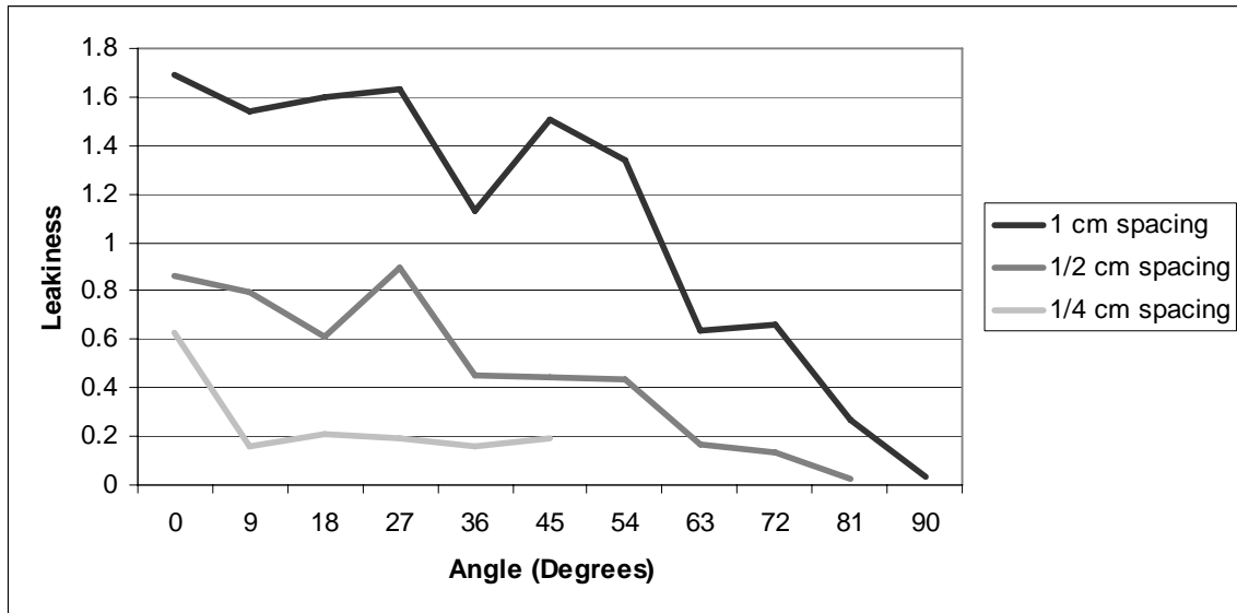
Fig. 6. Leakiness as a function of angle in 9 degree increments from 0° to 90°, for Re .047.
