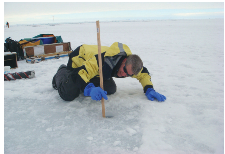
Ken Golden measuring the fluid permeability of sea ice. Photo credit: Adam Gully
