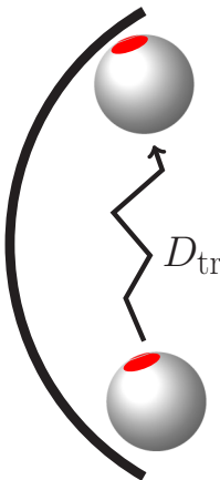
FIG. 7. The thick black curve depicts a curved absorbing left wall. Here (35) is not satisfied, and the wall curvature affects the patch orientation relative to the wall.
